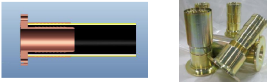
Figure 2: Land RTP connection structure diagram Steel connector
