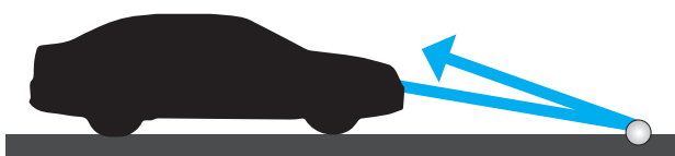
With light reflecting glass beads.
